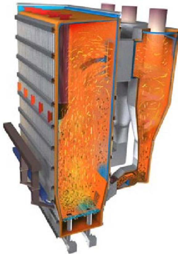
Figure 3.21 CFB process shown schematically
