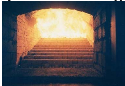
Figure 3.10 Picture of an inclined moving grate
