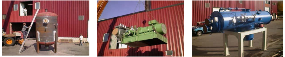
Figure 6.16 Equipment before erection: flash-box, turbine and vacuum condenser respectively
